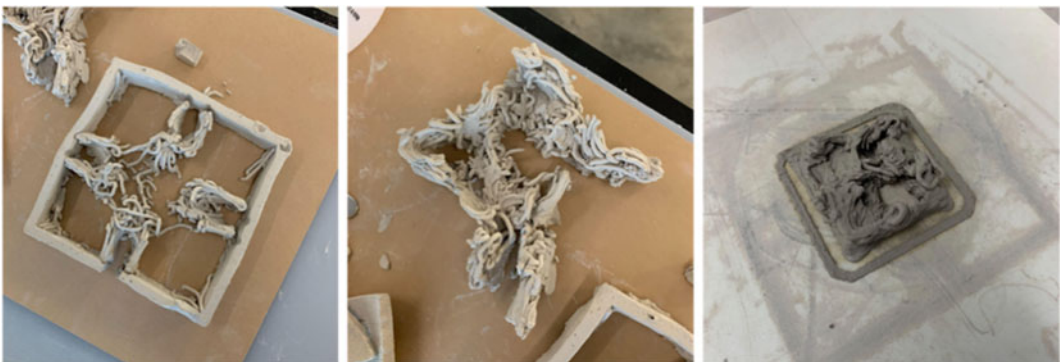
Fig. 47.16 Early trial clay prints using GCODE automatically generated by the slicer
