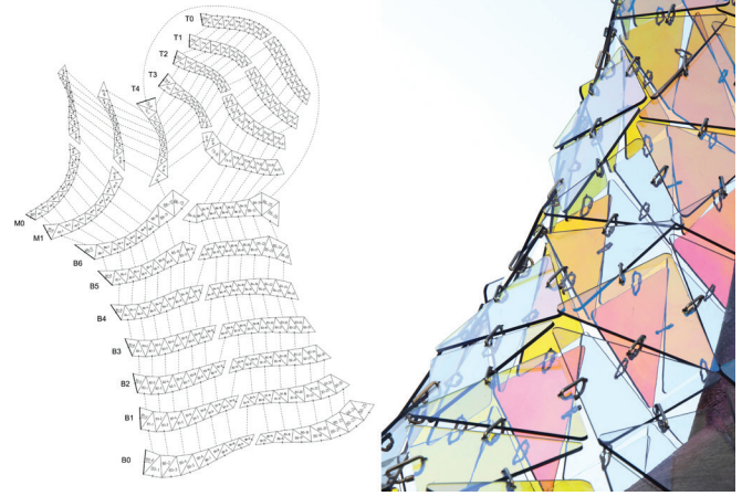
7 To fabricate the panels, 0.75" polycarbonate flat sheets were laminated with wavelength dependent dichroic film and cut via CNC process
