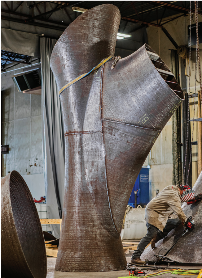
9 Attempts were made to remove the presence of visible arc start locations through grinding, but it was determined that this would create noticeable grind patches; due to labor, cost, and time, the ribbed texture with periodic bumps provided a beautiful texture and narrative of its robotic wire arc production
