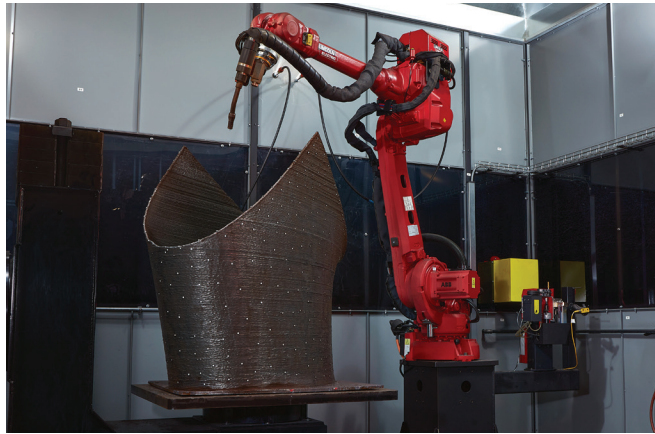
6 Section C of the project being printed in a cell at Lincoln Electric; BLUE MAX® MIG 316LSI was used to additively manufacture each of the nine 0.25" thick parts via Wire Directed Energy Deposition (Wire DED) on a 0.5" thick ASTM A36 base plate; the method of DED was GMAW-Pulse
