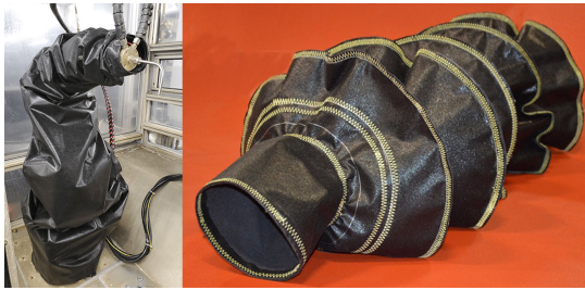
Figure 3: Robotex protective covering for robotic arms (Source: Gretchen Reimbold - Mid-Mountain Materials)
